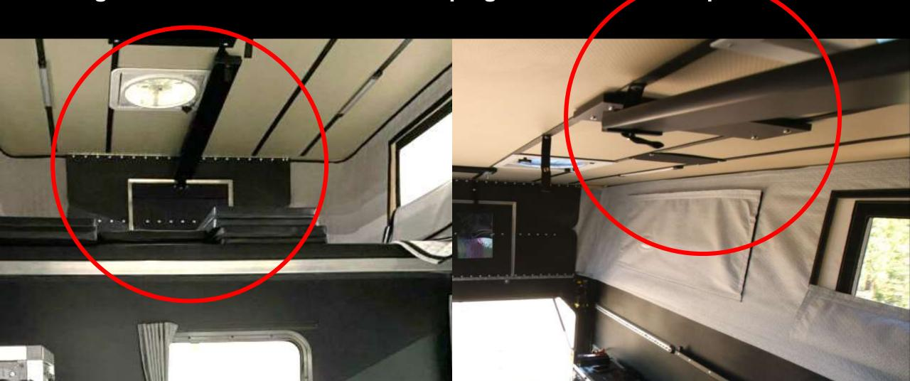
This thin, composite board is what supports the weight of the roof.
