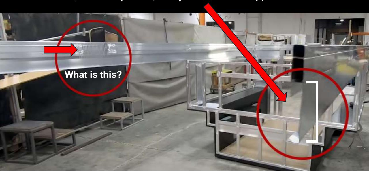
This is how they form their Radius "Structure" - by Notching their Thin Aluminum Tube and C-Channel every  $\frac{1}{4}$ " so they can bend it.
