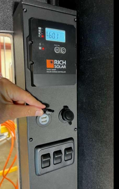
Each OV-X features our custom-designed Soaring Eagle Electrical Center which is hand-crafted out of sturdy composite material. This handy set up separates us from the competition as it neatly houses the solar panel control system, 12V outlets (including USBs) and also has the light and fan switches which are easily reached from outside the camper.
